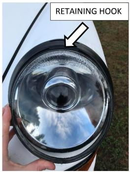
11) Remove the previously installed headlight retaining screw. Install the trim ring over the headlight frame. Start at the top of the trim ring and push the trim ring down over the headlight frame until the screw hole at the bottom lines up with the headlight bucket threads.
