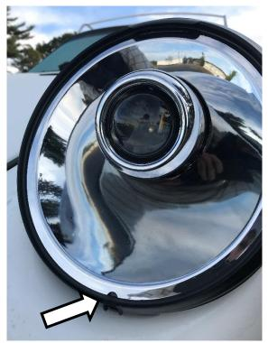
9) Install the supplied lens gasket to the supplied lens. Stretch the gasket over the edge of the lens. Be sure the ribs of the gasket face away from the lens.
