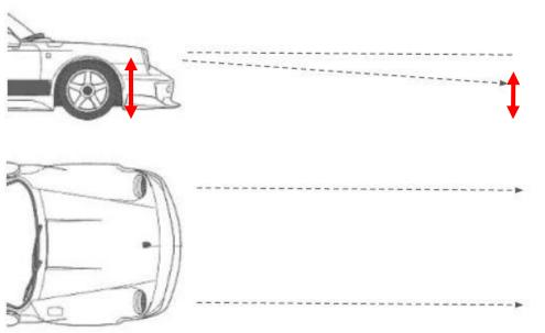
The upper cutoff shadow line with low beams should be 2" lower than the height of the projector from the ground when measured 25' from the vehicle. This measurement is easily taken with the vehicle parked 25' from a wall, measuring the cutoff line on the wall.
