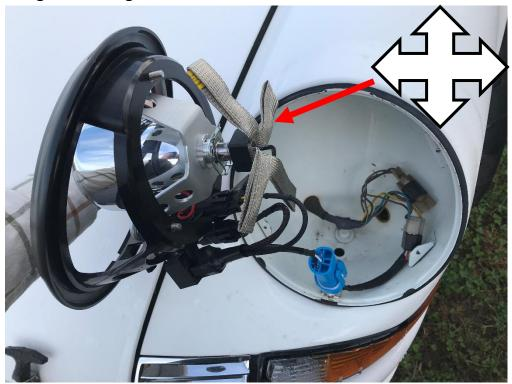
5) Align the top of the headlight assembly, marked by the arrow on the headlight frame, to the top of the fender's headlight bucket. Hook the lip of the headlight over the lip of the fender's headlight bucket.
