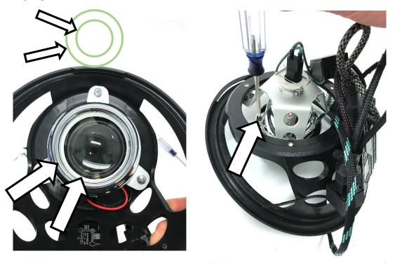
3. Secure the LED power module to the headlight frame using the supplied zip tie. Secure the excess wires using the supplied wire clamp and screw, screwing the wire clamp to the body of the headlight frame.
