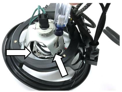
1. Install the Angel LED into the projector shroud. Orient the wires to the bottom of the shroud. The bottom is designated by the screw mounting locations that are further apart.
